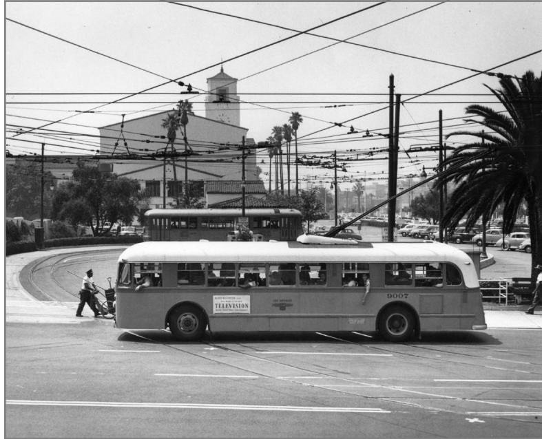
Pacific Electric Bus powered by electricity and driven on tires not tracts.
